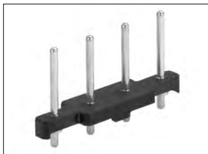
4-contact male header for THR-soldering; grid 5.75 mm
